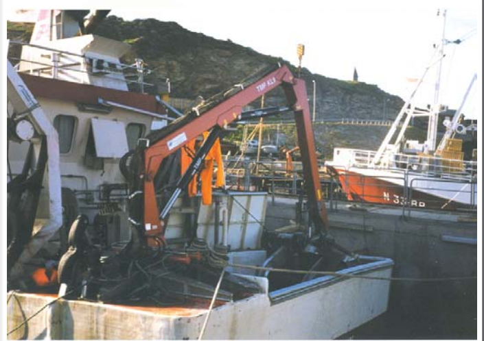
Meydam TMP KL 9 with T 1300 stacker head.
